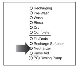
■ When the "Neutralizer" indicator comes on, it is important to promptly refill or exchange the neutralizer container.
